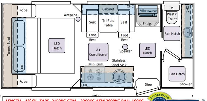
LENGTH - 18' 6" TARE -2150KG GTM - 2360KG ATM 2600KG BALL-160KG
